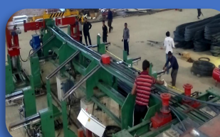
Rebar Bending m/c
