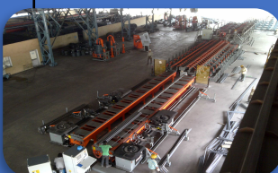
Rebar Cut & Bend m/c
